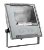
Floodlight in die cast aluminum with galvanized bracket and painted the same color as the body. Equipped with graduate scale to facilitate orientation. Flat tempered glass 4 mm thickness silk screen printed; hinged to the body for quick access inside the Floodlight. Anti aging silicone gasket. Power input through PG13.5 for cables Ø 6.5 ÷ 13 mm. Optic in 99.85% polished and anodised aluminium. Electrical componenent plate in galvanized steel. Quick wiring tripolar terminal block.
