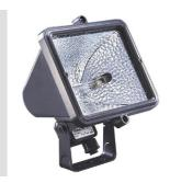
Multifunctional floodlights in die-cast aluminium, painted with polyester powders, for fixed applications. Optic in 99.85% polished and anodised aluminium. Flat tempered glass 5mm thickness. Anti-aging silicone gasket. Suitable for use with halogen lamps. Power input through cable gland for cable Ø 9÷12 mm.
