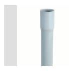
The system of medium rigid protective conduits made of high quality PVC to offer superior performance. Available in diameters from 16 to 32 mm and in lengths from 2 to 3 m. They can be integrated with flexible conduits and junction boxes. Completing the offer, a wide range of couplings and routing components with IP40 and IP67 degree of protection.
