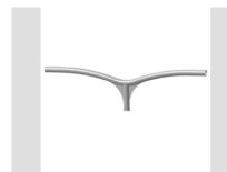
Double pole head bracket in hot galvanised steel tubing, 3 or 4mm thick, hot galvanised steel and painted with polyester powder. Supplied with three M8 stainless steel lockscrews for fixing on poles of 60mm diameter.
