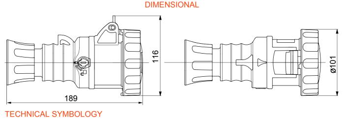
IP IK 125 °C (active parts) 1P66/IP67/IP68/IP69 IK09 -25 +55 °C With screw With screw Balogen-free in compliance with EN -650 °C (passive parts) -80 °C (passiv
