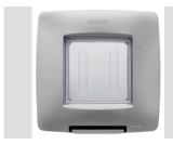
Watertight plates IP55 ChoruSmart range for round/square (axles distance 60mm) and rectangular (3 and 4 modules) flush mounting boxes. Watertight plates equipped with support and long screws, for the installation of Chorusmart range devices. Ergonomic membrane, maximum opening angle lid 160° facilitated by a comfortable handle. IP55 degree guaranteed with closed lid and watertight plate mounted on smooth and waterproof walls, without grooves
