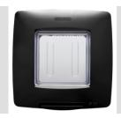
Watertight plates IP55 ChoruSmart range for round/square (axles distance 60mm) and rectangular (3 and 4 modules) flush mounting boxes. Watertight plates equipped with support and long screws, for the installation of Chorusmart range devices. Ergonomic membrane, maximum opening angle lid 160° facilitated by a comfortable handle. IP55 degree guaranteed with closed lid and watertight plate mounted on smooth and waterproof walls, without grooves
