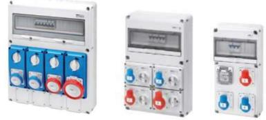
In places where maintenance and process work is carried out with mobile or portable electric tools, plug socket distribution boards must be used, located so as to avoid that the flexible cables or stretcher cords are excessively long (a distance of not more than 15-20m is recommended between the distribution boards, in the whole working area). The choice and size criteria are summarised in the figure. In particular, the following characteristics are highlighted:
