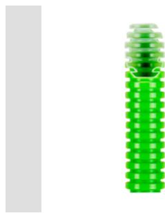
FK-Xtreme is a series of folding tubes available in 4 diameters (from 20 mm to 40 mm) and 6 colours, to identify the different lines of the electrical system. FK-Xtreme tubes are made via a co-extrusion process, which prevents the infiltration of liquid cement used for the creation of self-levelling substrates and allows the mechanical properties of the tubes to remain intact, even in extreme conditions. The range is designed to facilitate optimal setting and wiring operations.
